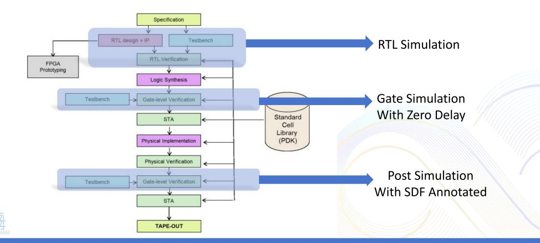
RTL-Sim focus on RTL functional issues, Only Post-Sim carry the exact timing delay information
