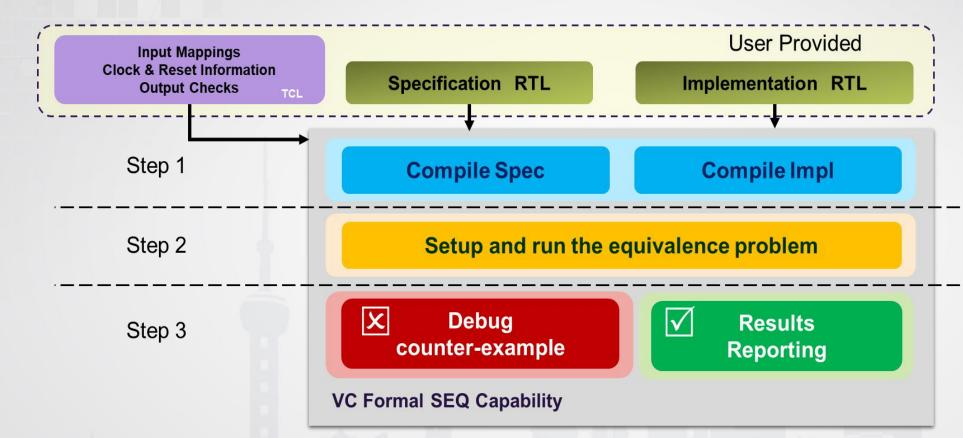
Two designs that produce same output on every clock cycle from valid initial states given the same inputs are sequentially equivalent.
