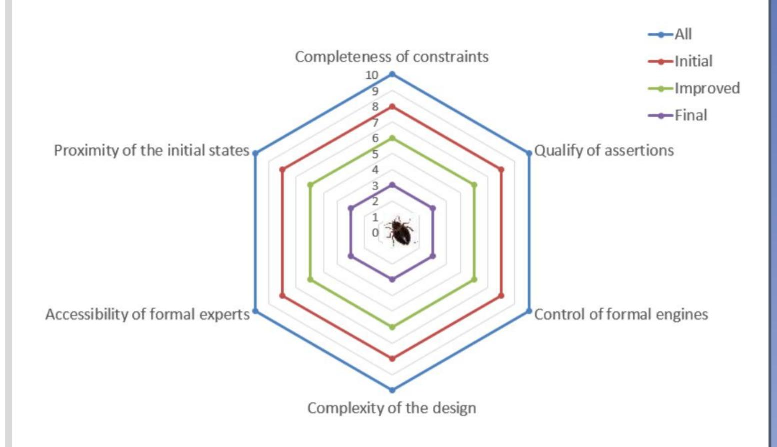
The radar chart guides the deployment of formal verification to find deep silicon bugs Phase 1: "Initial"
